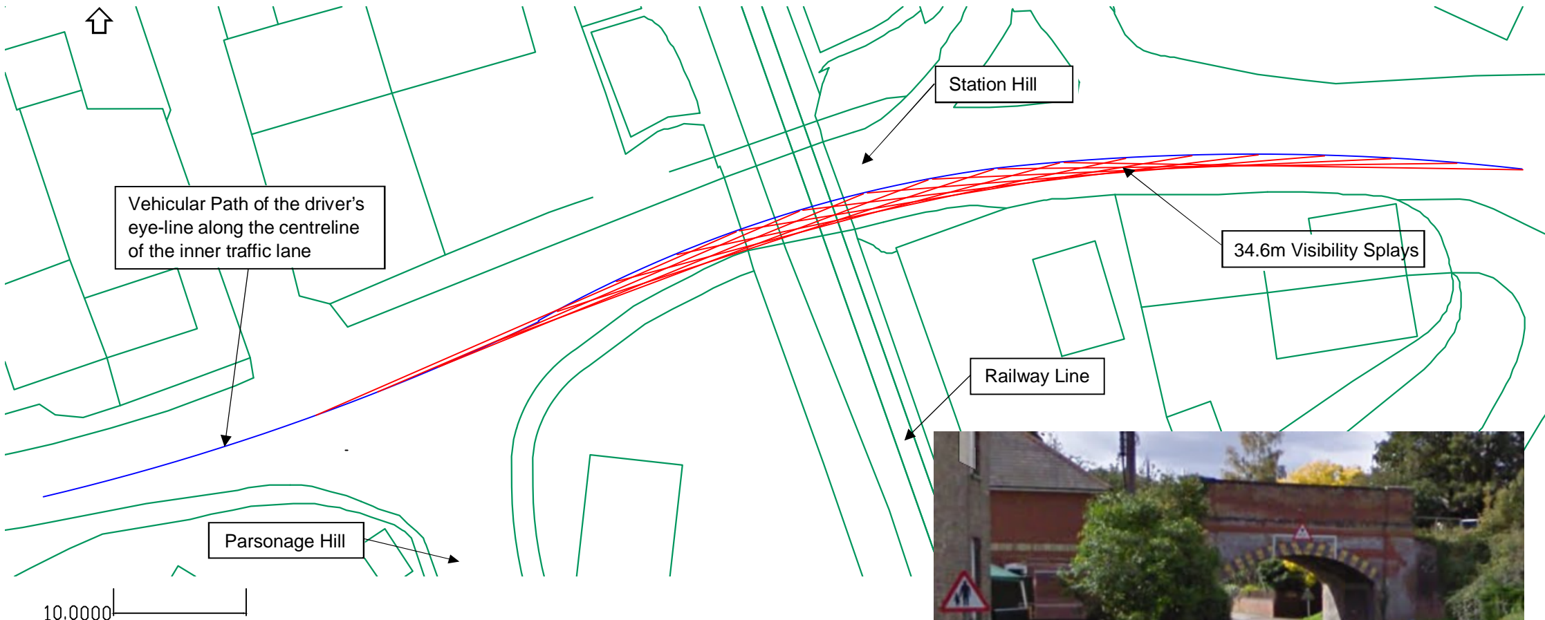
Figure 3: Plan view of visibility splays on Station Hill and view looking westbound from the east side of the railway
