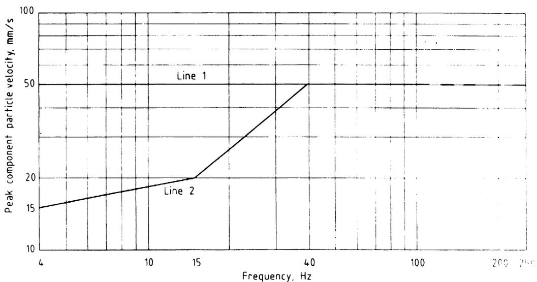
Figure 1 — Transient vibration guide values for cosmetic damage
