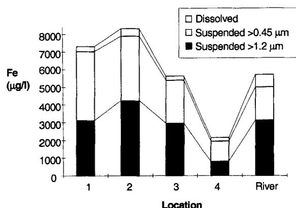
Fig. 3. Partitioning of iron between dissolved and particulate forms, Pond C (April 1999)
