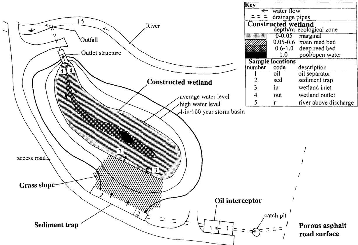
Fig. 1. Diagram of Pond C showing typical design features and sampling locations
